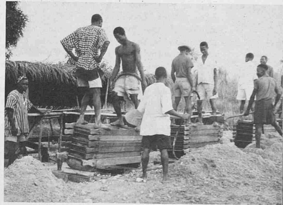
A prospecting team uses foot jigs to size gravel which has been taken from the prospecting pits
